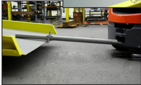
The "Tow Clamp" connects between the ramp pocket and the tow hitch of your fork truck and permits easy transportation of the lift over longer distances.
